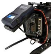
**Quick media change.** Flip up the V-Lock battery for fast CFast swap on the ARRI Mini.
