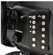
**User-assignable controls** for direct access to white balance, frame rate and many others.
