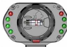
**Mirrored Light Level and Fuel Gage indicators** provide at-a-glance reading from either side.
