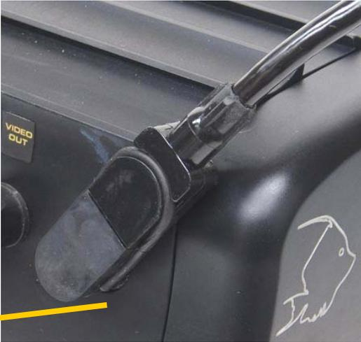
6 pin connector mated and secured with retainer strap
