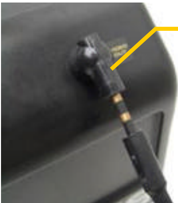
Plug in the EM419 cable to the bulkhead connector. (HD1 housing shown)
