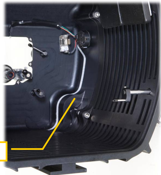
Typical Water Alarm installation.
