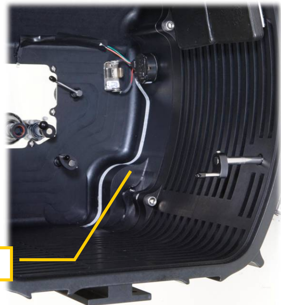
Typical Water Alarm installation.
